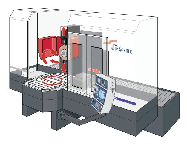
Like its sister systems in the MFP series, the lows loading and unloading of workpieces while and unloading system, the MGC with swivelling MÄGERLE Grinding Center delivers superb re- machining is in operation. Non-productive times table frees up additional resources. The openly sults for creep feed grinding as well as for pro- for workpiece change are thus largely eliminated. accessible swivelling table also provides the file and surface grinding. In its swivelling table
